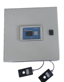
BMSL monitoring system monitors and signals in the real time states of accumulator batteries, for example deep battery discharge, eventually discharging of single cells of the battery set, cell voltage unbalance, excessive discharging or charging currents of the battery set, battery temperature variation from the stated value and other parameters. Overrun of every mentioned parameter can destroy of the battery set, so it is needed to have immediate information about battery status.
