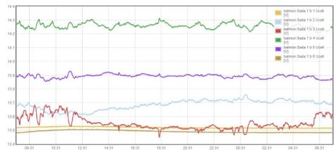
The graph below displays the same battery string after applying Equalization of voltage in cells. As evident from the graph, BMSV can equalize these cells over a few hours and therefore extend their lifespan.
